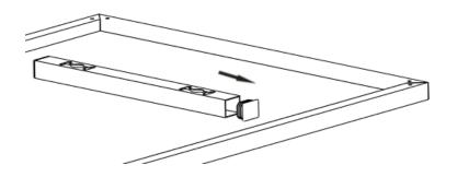
4. Slide the panel onto one side of the panel's rear brackets first, then push the whole panel close to ceiling and slide the panel back, to make sure the "ends" of other end of the ceiling hanging bars enters the other side.
