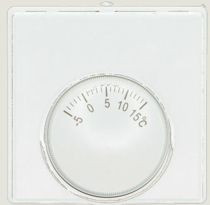
Designed for wall mounting, with 60mm fixing centres for back-box compatibility, and suitable for in-wall or surface-run wiring connection. The thermostat cover incorporates four breakouts for surface-run conduit. The temperature regulation mechanism is the well-proven sealed bellows system. Install in parallel to the room thermostat in a cool area of the property, to protect the property, heating system and boiler against the risk of damage from frost.
